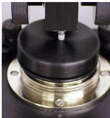
ATR accessory pressed at functional pressure on ATR Validation Standard.
