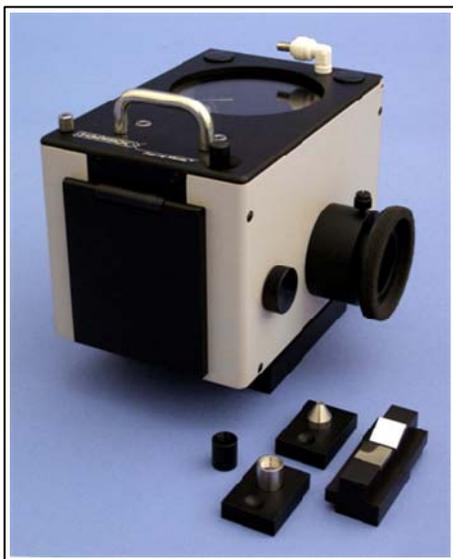
Figure 1. The Praying Mantis Diffuse Reflectance Accessory.
