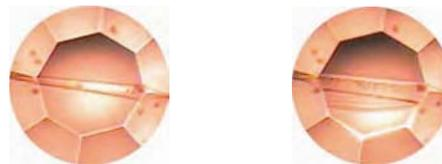
Figure 2. Photographs of the 20  $\mu\text{m}$  PET Fiber compressed with 20 (left) and 302 (right) units of pressure.
