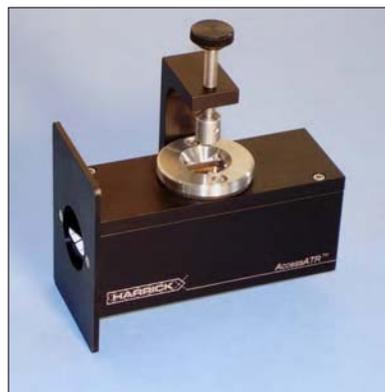
Figure 3. AccessATR single reflection ATR accessory.
