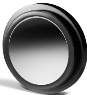
Specular Reflectance Standard – for calibrating reflectance measurement system
