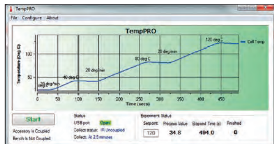
TempPRO software for graphical setup and control of kinetic measurements.
